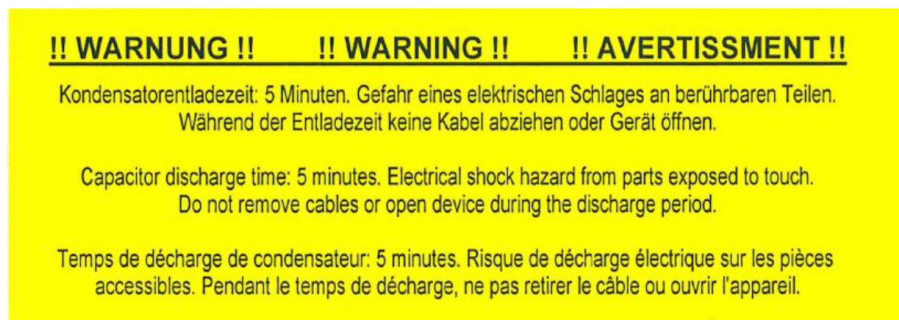
Figure 1: Warning label for capacitor discharge period
